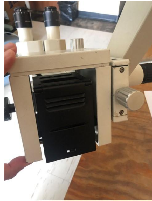
(4) OEM lamp house from back side.
