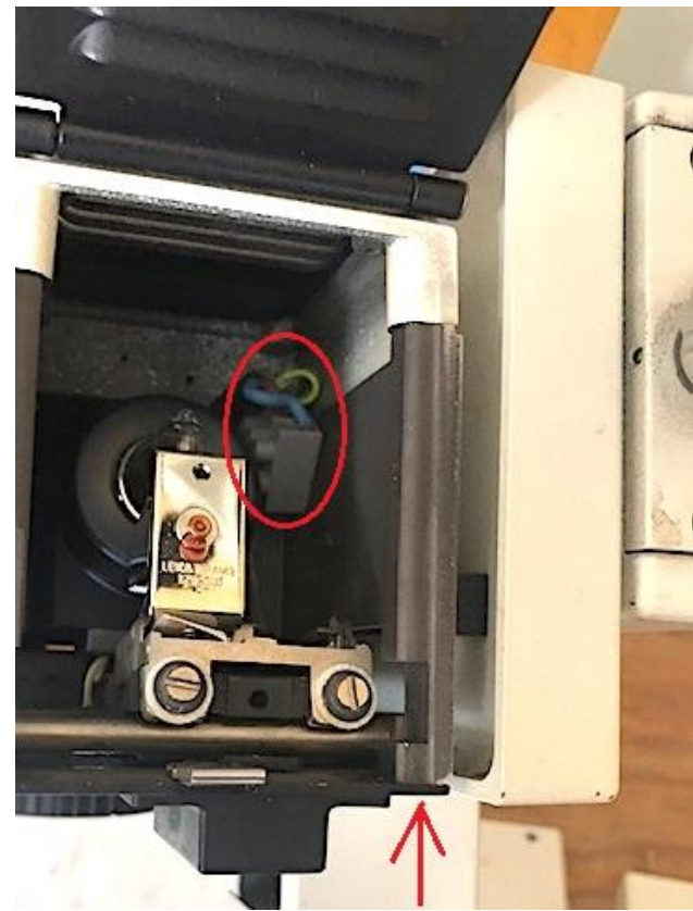
(6) Power cord, red circle. Mounting screws, 1 of 4, red arrow.
