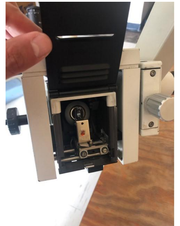
(5) Back cover lifted, lamp holder visible.
