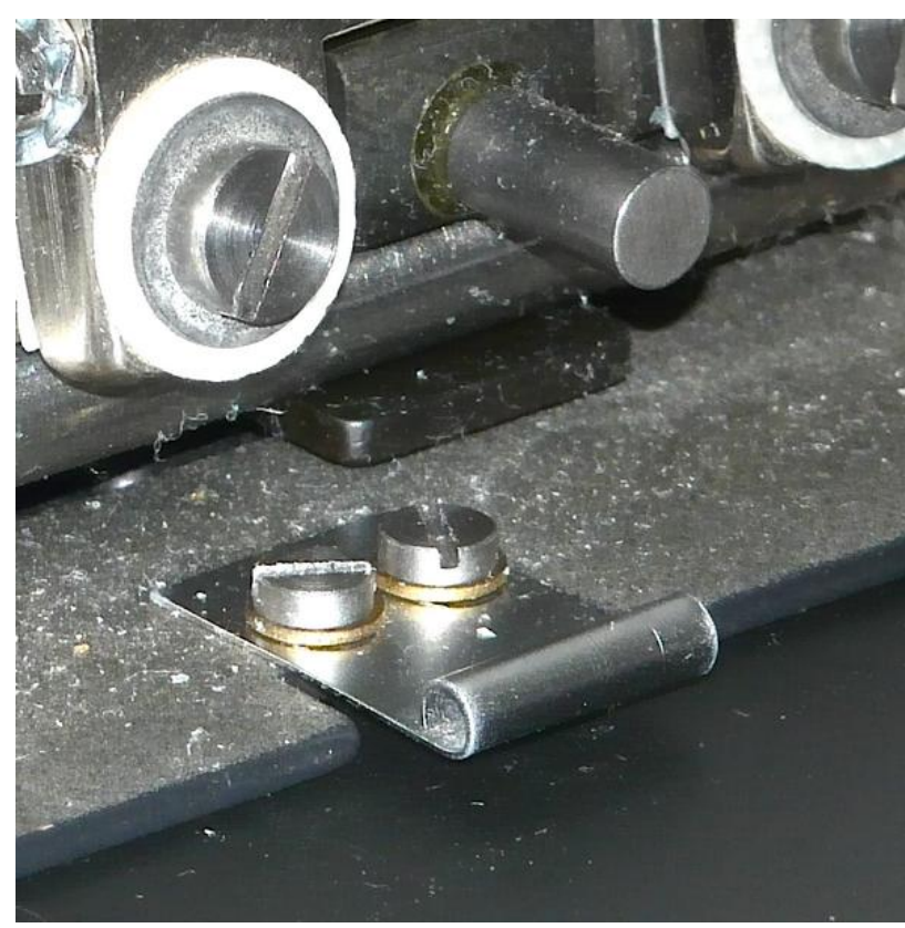
(8) Close up of latch (to be removed). Circled in red, photo at left.
