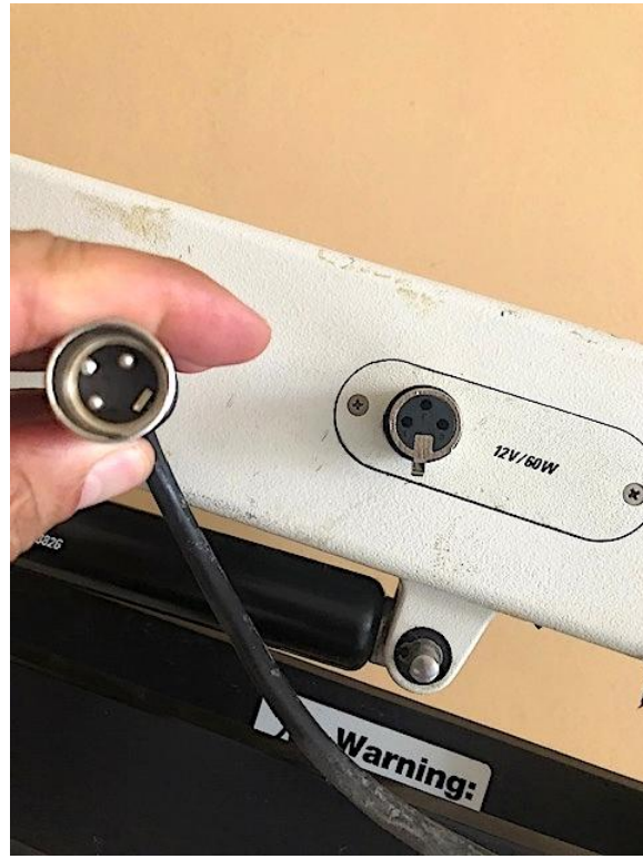
(3) Lamp power cable.
